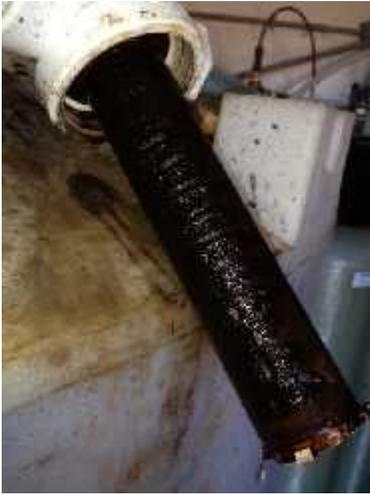
**LEFT** - This is what a small simple filter looked like with the chlorine treatment. The water flowing through this small filter was filtered first by large iron eating filters.
