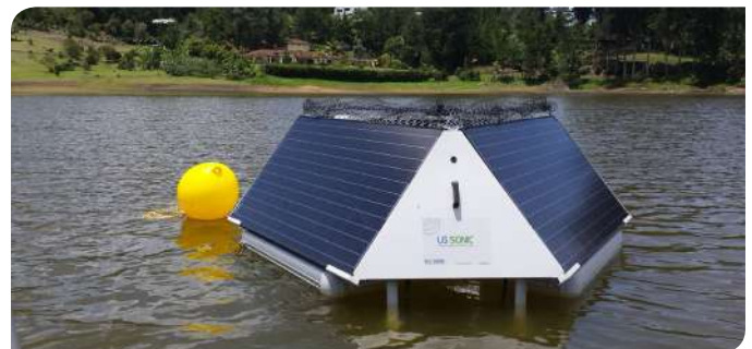
Figure 1: Close-up of the MPC-Buoy installed in La Fe reservoir
