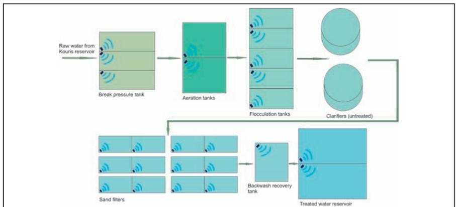
Figure 2: Overview of the Limassol Water Treatment Plant and where LG Sonic Devices were Installed
